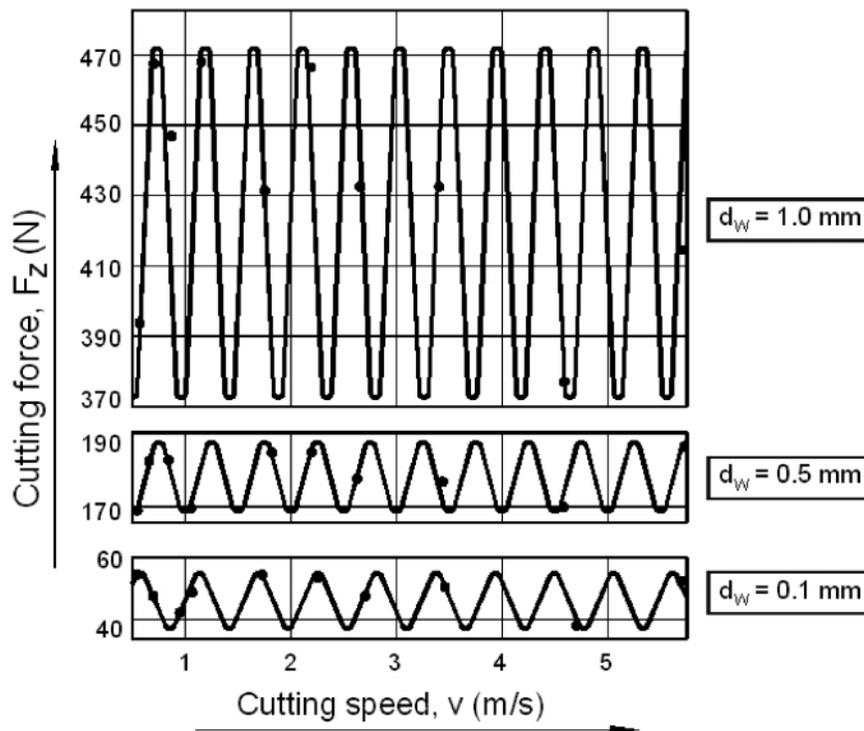
Figure 5: Experimental Results Represented as Sinusoidal Periodic Data in the Coordinate System “v – F<sub>z</sub>”.
