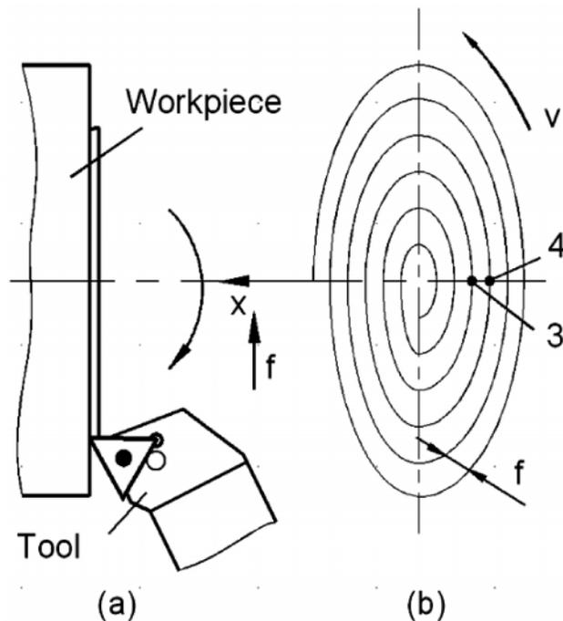
Figure 8: (a) Face Cutting and (b) The Trajectory of the Cutting Tool
