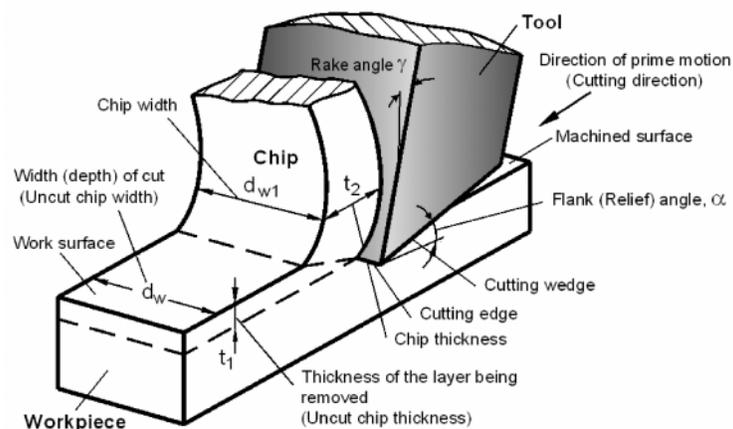
Figure 1: Components of the Cutting System
