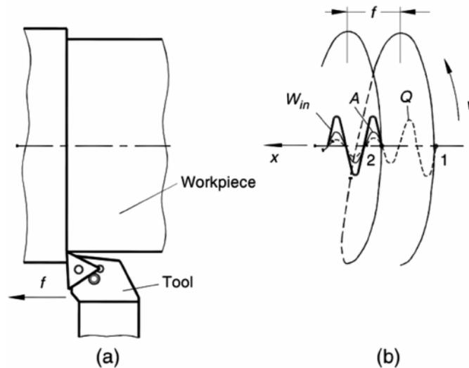
Figure 4: (a) External Bar Turning and (b) The Trajectory of the Cutting Tool
