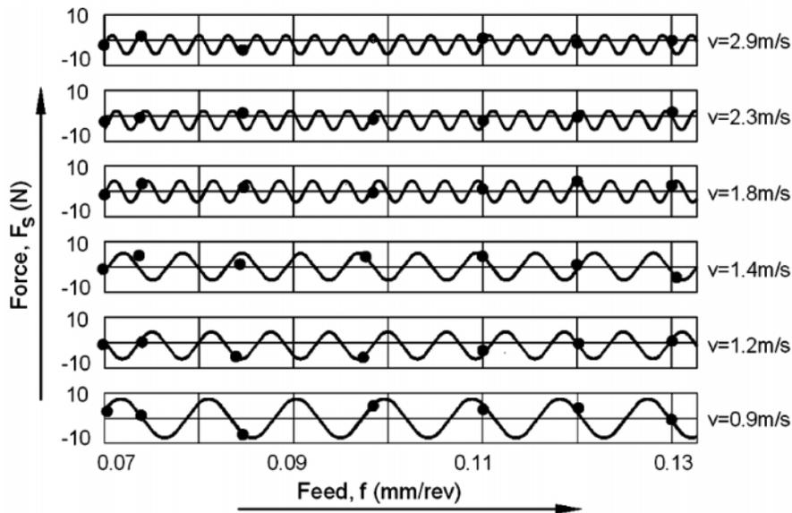
Figure 9: Sine Wave Approximation of the Experimental Data in the Coordinate System “ $f - F_z$ ”
