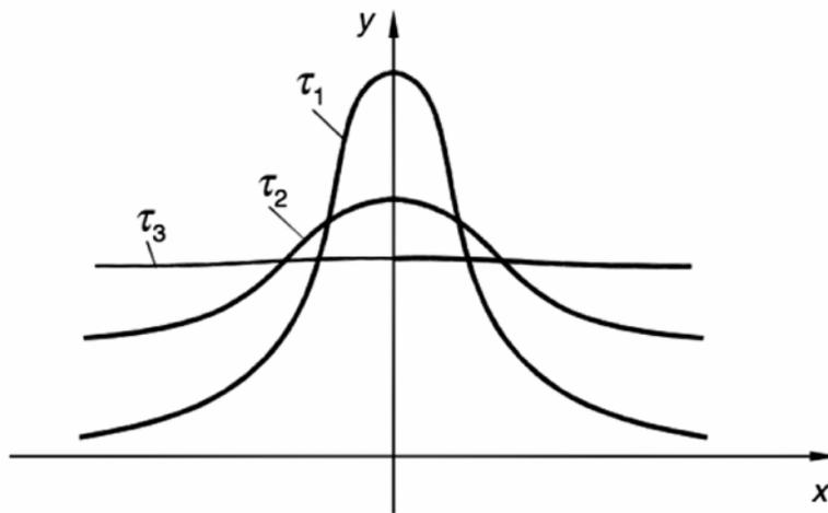
Figure 3: Intensity of a Decaying Heat Source
