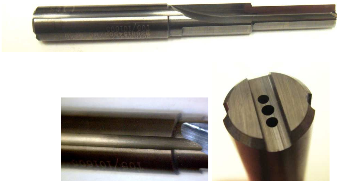
Figure 4. Slots-coolant passages made on the shank to provide the coolant to the chamfering part of the tool
